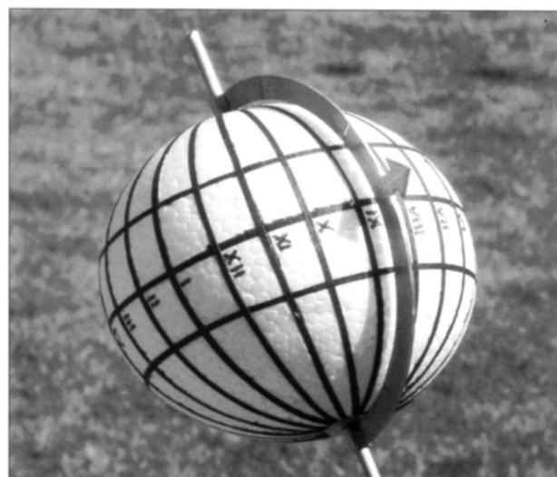
Fig 6. Model of Sphere with moving Gnomon.
