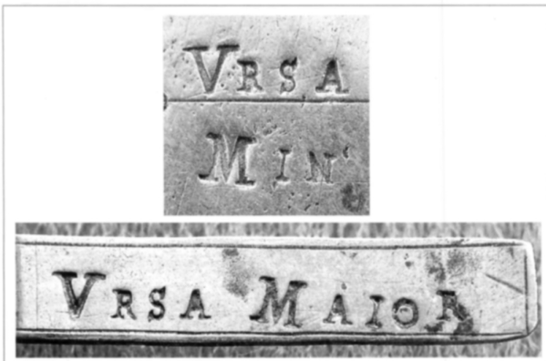
Fig.6. Punch marking from two parts of a brass Nocturnal. Note that the same punches were used for both inscriptions. In particular, note how the enclosed part of the A is filled in, probably due to a clogged punch.
