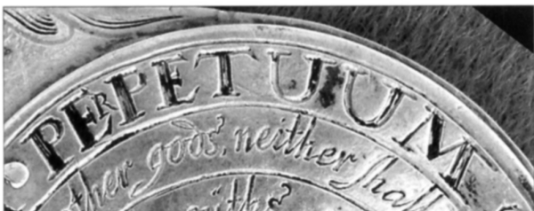
Fig. 4. An engraving error from a silver Perpetual Calendar. the R was missed in the word PE R PETUUM and has been fitted in later.
