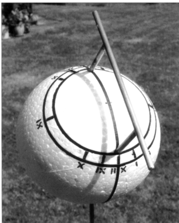
Fig 7. Polar Dial Mounted on a Sphere.
